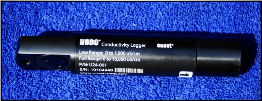
Conductivity Range (low setting):  $0 - 1,000 \mu$ S/cm Accuracy: 2%  $0 - 1,000 \mu$ S/cm
