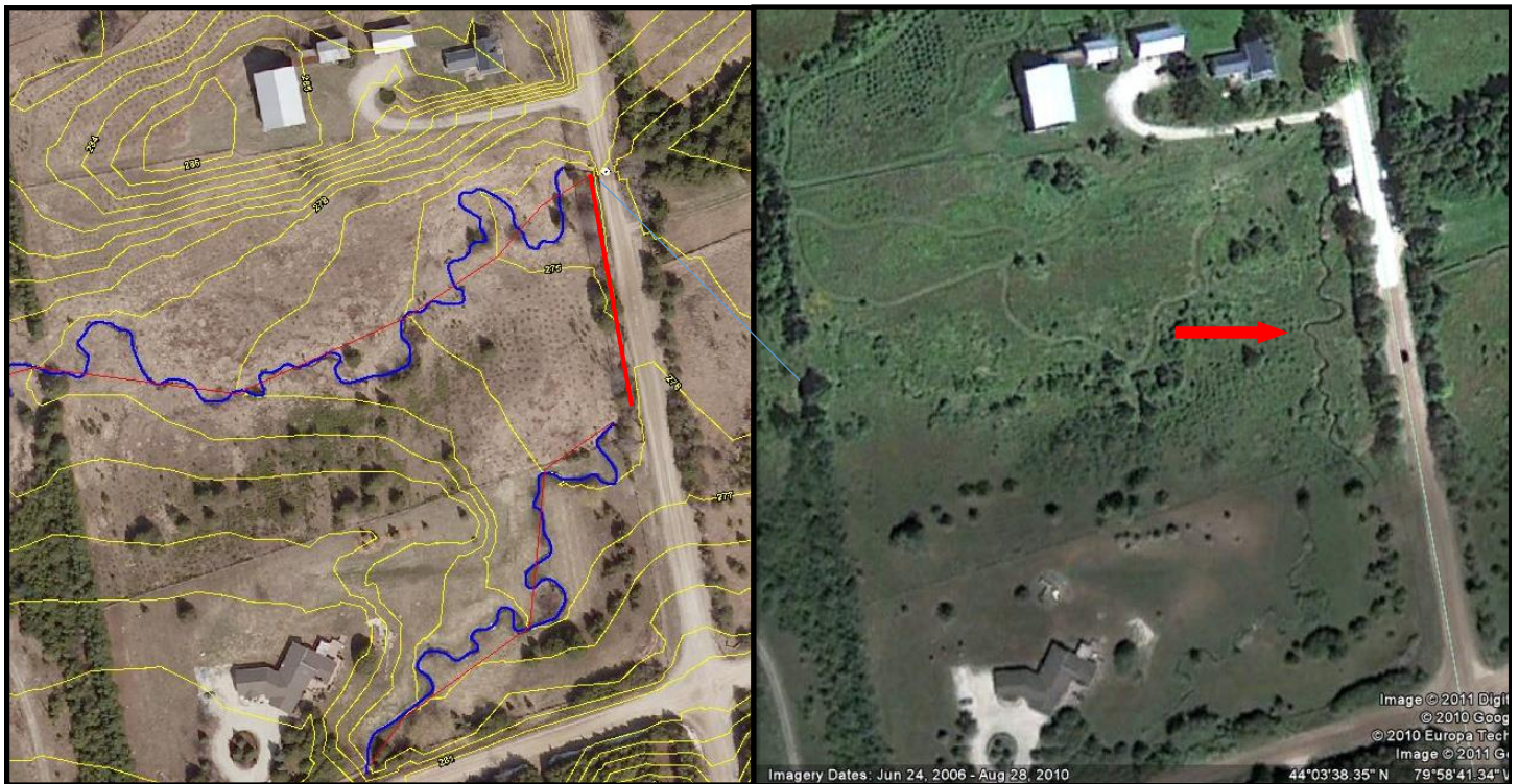
Left photo shows pre-construction condition and existing streams with channel along road (red line); Right photo shows meandering natural stream channel as completed.
